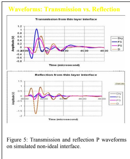
Figure 5: Transmission and reflection P waveforms on simulated non-ideal interface.
