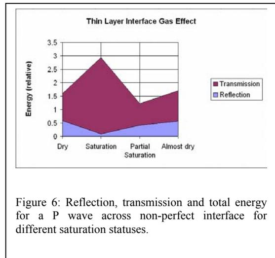
Figure 6: Reflection, transmission and total energy for a P wave across non-perfect interface for different saturation statuses.
