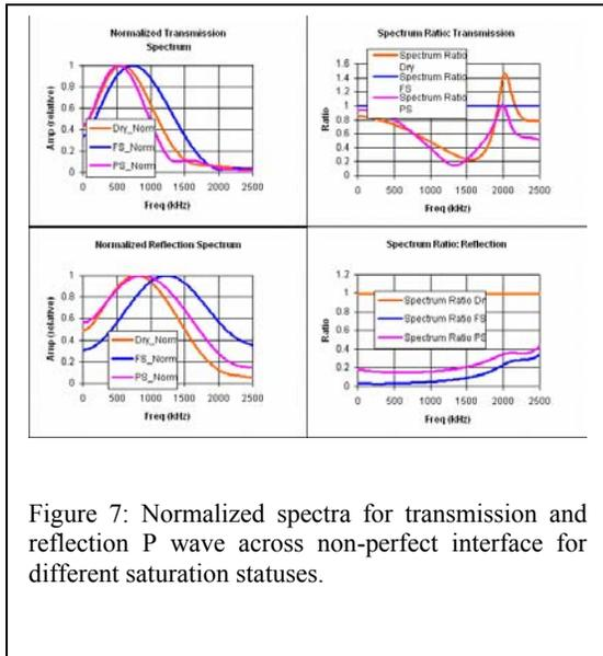
Figure 7: Normalized spectra for transmission and reflection P wave across non-perfect interface for different saturation statuses.
