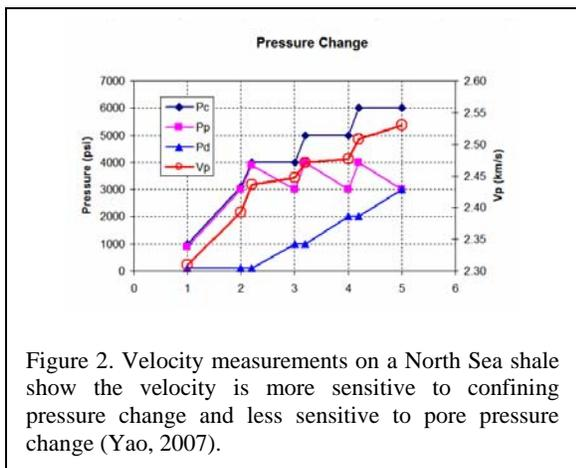
Figure 2. Velocity measurements on a North Sea shale show the velocity is more sensitive to confining pressure change and less sensitive to pore pressure change (Yao, 2007).
