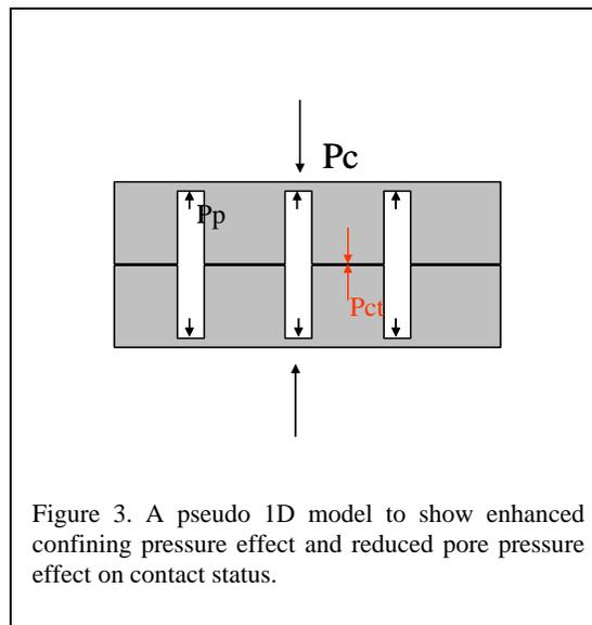
Figure 3. A pseudo 1D model to show enhanced confining pressure effect and reduced pore pressure effect on contact status.
