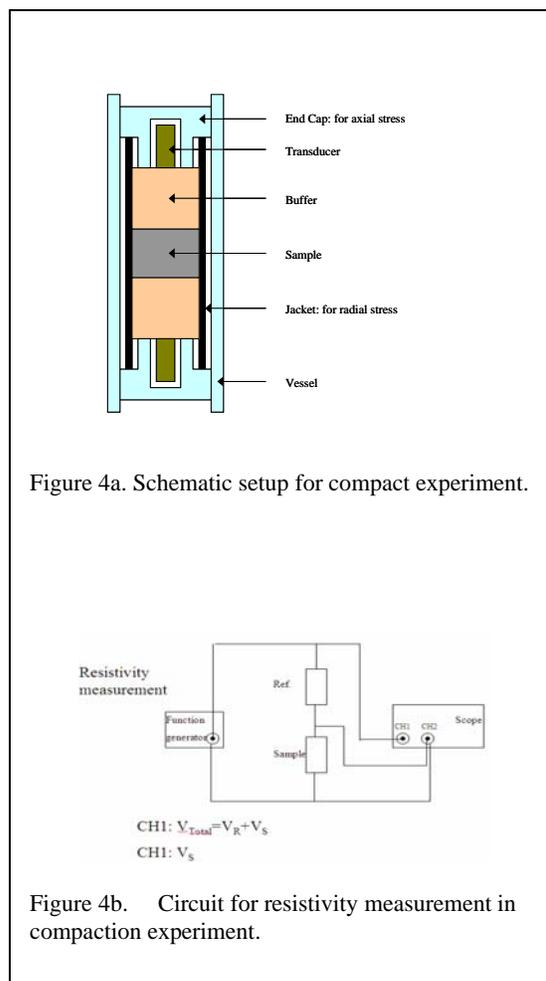
Figure 4a. Schematic setup for compact experiment.
