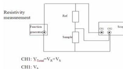
Figure 4b. Circuit for resistivity measurement in compaction experiment.
