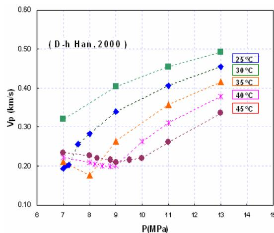
Fig.3 Measured velocities of CO<sub>2</sub> as a function of pressure P for the range near the CO<sub>2</sub> critical point.
