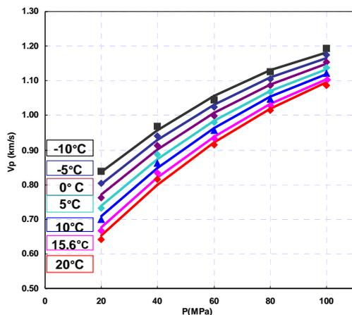
Fig.4 Calculated (solid lines) and measured velocities of CO<sub>2</sub> as a function of pressure P for different low temperatures from 20 °C down to -10 °C.
