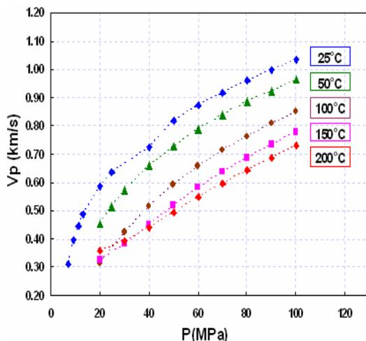
Fig.2 Measured velocities of CO<sub>2</sub> as a function of pressure P for different temperatures from 25 °C up to 200 °C.
