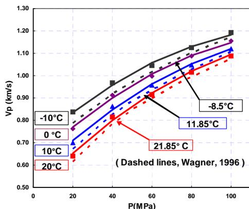
Fig.7 Comparing the calculated (solid lines) and measured velocities with the calculated velocities (dashed lines) by Span and Wagner for the low temperature and high pressure range.
