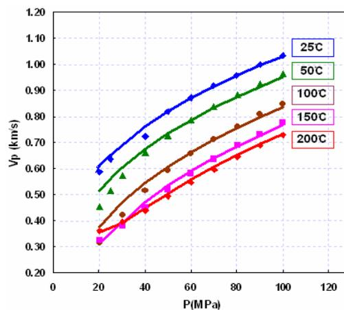
Fig.5 Calculated (solid lines) and measured velocities of CO<sub>2</sub> as a function of pressure P for different temperatures from 25 °C up to 200 °C.
