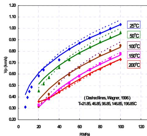
Fig.8 Comparing the calculated (solid lines) and measured velocities with the calculated velocities (dashed lines) by Span and Wagner for the high temperature and high pressure range.
