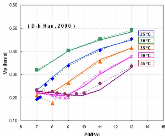
Fig.6 Calculated (solid lines) and Measured (dashed lines) velocities of CO<sub>2</sub> as a function of pressure P for the range near the CO<sub>2</sub> critical point.
