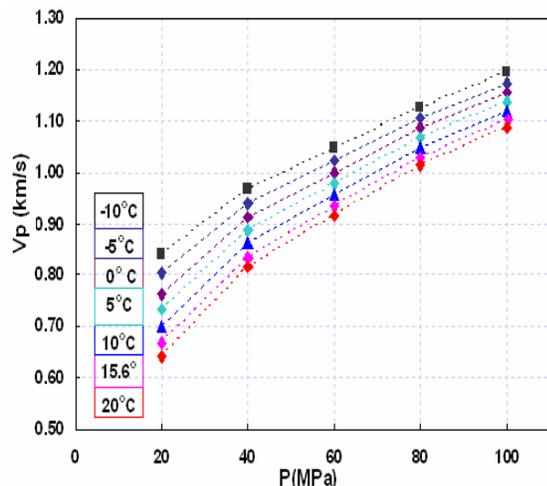
Fig.1 Measured velocities of CO<sub>2</sub> as a function of pressure P for different temperatures from 20 °C down to -10 °C.
