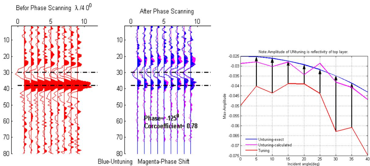
Figure 4 Seismic responses with random noise of  $S/N=2$  for tuning thickness and zero phase Ricker wavelet. Left: tuning response; Middle: Un-tuning response (blue) and calculated data (magenta); Right: extreme of amplitude of each trace from corresponding seismic responses (see colors). The most Fitting data is obtained when correlation coefficient equal to 0.78, and addition phase here is  $-125^{\circ}$ .
