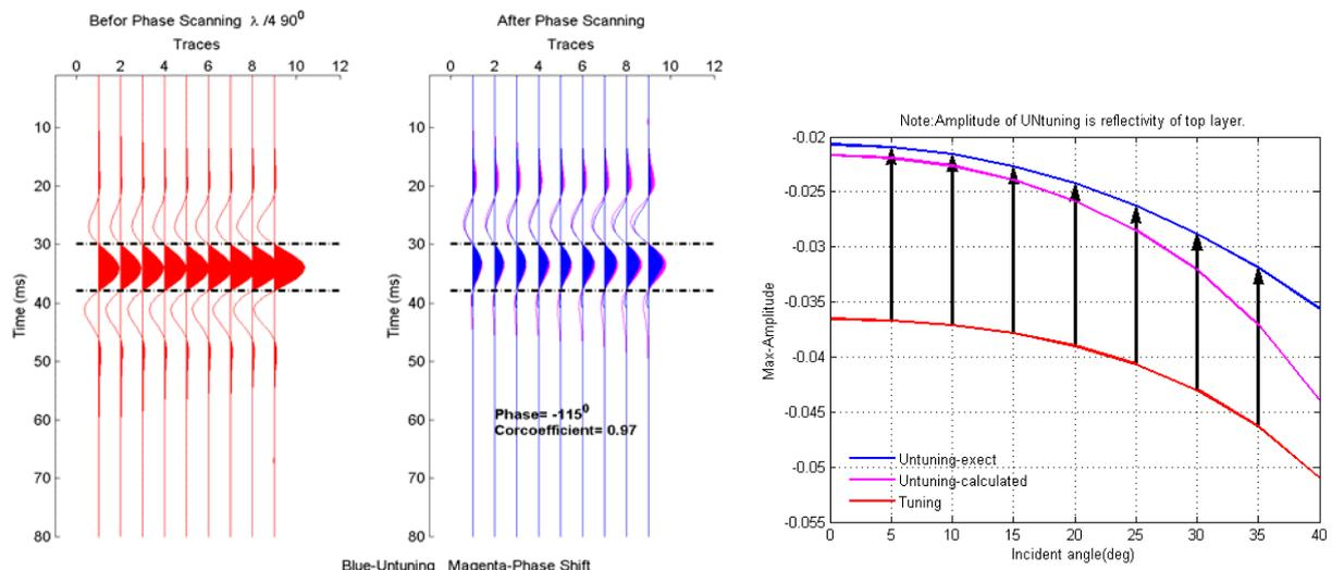
Figure 3 Seismic responses for the case of tuning thickness ( $\lambda / 4$ ) and  $90^{\circ}$  phase Ricker wavelet. Left: tuning response; Middle: Un-tuning response (blue) and calculated data (magenta); Right: extreme of amplitude of each trace from corresponding seismic responses (see colors). The most Fitting data is obtained when correlation coefficient equal to 0.97, and addition phase here is  $-115^{\circ}$ .
