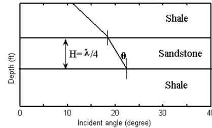
Figure.1 Thin bed model (incident angle between  $0^\circ$  and  $40^\circ$ .)
