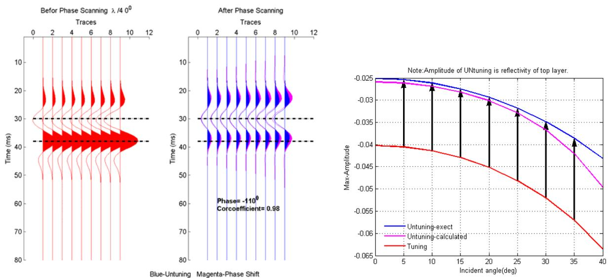
Figure.2 Seismic responses for the case of tuning thickness ( $\lambda / 4$ ) and zero-phase Ricker wavelet. Left: tuning response; Middle: Un-tuning response (blue) and calculated data (magenta); Right: minimum amplitude of each trace from corresponding seismic responses (see colors). The most Fitting data is obtained when correlation coefficient equal to 0.98, and addition phase here is  $-110^\circ$ .
