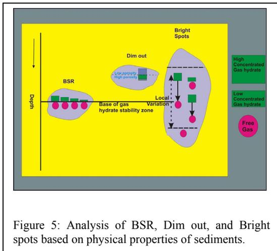
Figure 5: Analysis of BSR, Dim out, and Bright spots based on physical properties of sediments.
