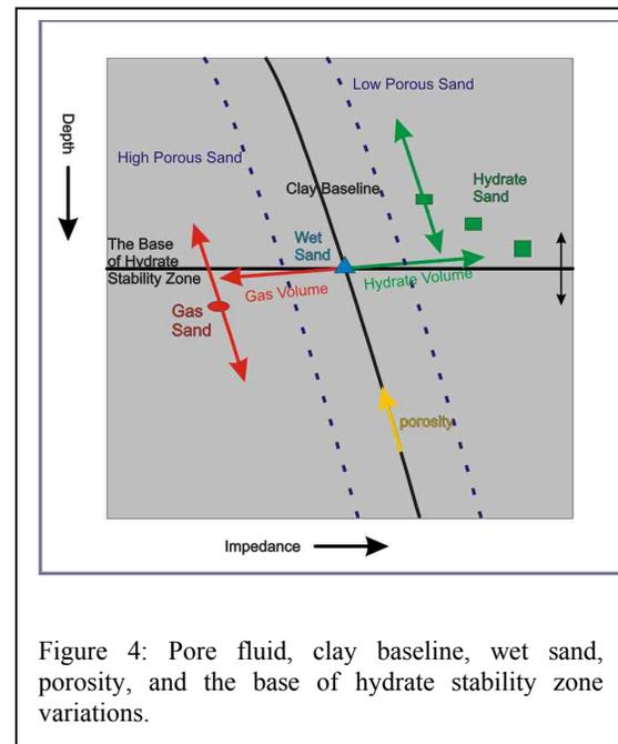
Figure 4: Pore fluid, clay baseline, wet sand, porosity, and the base of hydrate stability zone variations.
