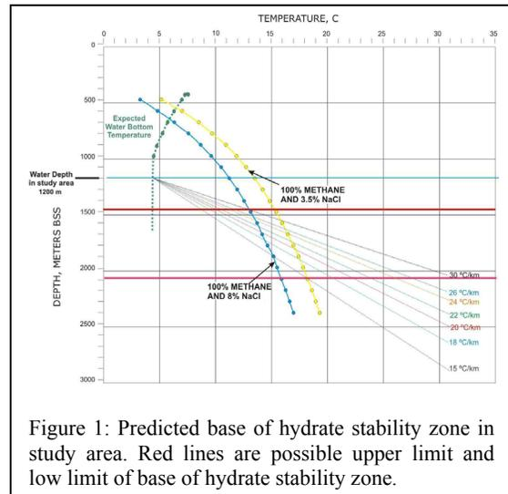
Figure 1: Predicted base of hydrate stability zone in study area. Red lines are possible upper limit and low limit of base of hydrate stability zone.
