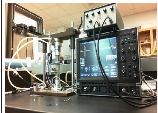
Figure 4: Ultrasonic velocity measurement setup
