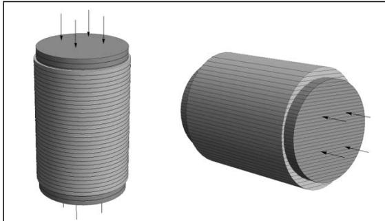
Figure 2 Schematic deformation of vertical plug(left) and horizontal plug(right) of VTI rocks under axial compression testing
