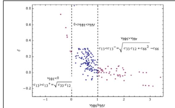
Figure 4: Crossplot between  $\delta$  and  $v_{HH}/v_{HV}$  ratio from dynamic velocity anisotropy measurement (137 of 203 data points are within the bounds)
