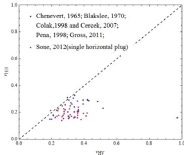
Figure 3: Static mechanic measurement of poisson's ratios on VTI rocks and rock-like materials.
