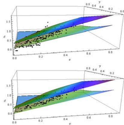
Figure 8: Comparison between measured and modeled ultrasonic velocities (above, all data; below, red data points in Fig. 4 removed).
